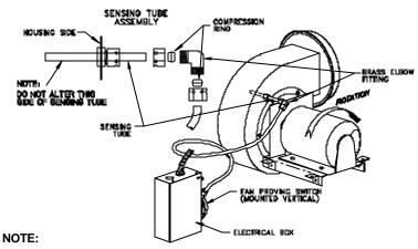
As viewed from the opposite end of the shaft, the motor should rotate clockwise
