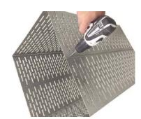
Locate the open edge of the box that has 2 holes near the edge of the corners. This open end of the box should face up for the next 2 steps. This is the bottom of the box. Install the (4) support brackets as pictured.
