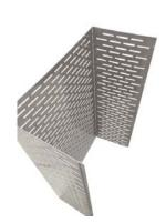
Align both formed panels with the offset edge on the inside of burning box. Using a drill with 1/4" nut runner bit and a 11/32" nut driver or wrench to hold nut on inside, install (5) of the 3/8" X 8-32 bolts and nuts down each of the 2 seems.
