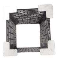
Locate the (4) Burning Material Support Brackets and form the tabs using a pliers as shown. Install the first (2) support brackets into the Box as shown using the holes furthest away from the feet. The (2) brackets are to be mounted side by side from each other and run parallel across the box.
