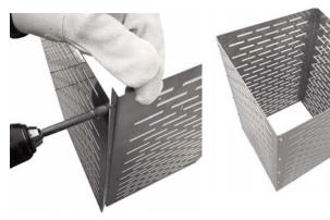
Locate the (4) feet and form the tabs on the feet as shown. The tabs should be formed up and should be about 90 degrees from the base foot.
