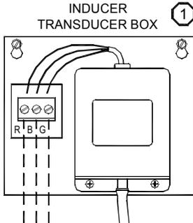
Route transducer wiring in metal conduit or use Belden Shield Cable #9939 or equivalent. Make sure the transducer wiring does not contain or cross line voltage wiring or undesired transducer performance may result.
