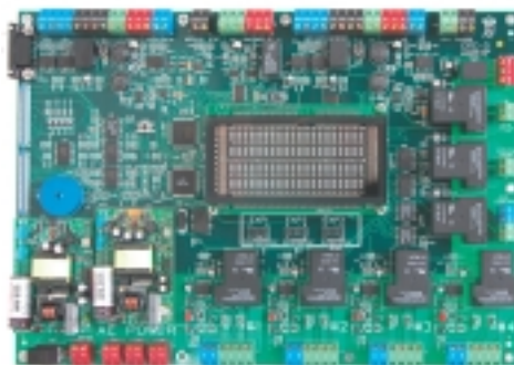
Circuit board inside CPC-3 Controller
